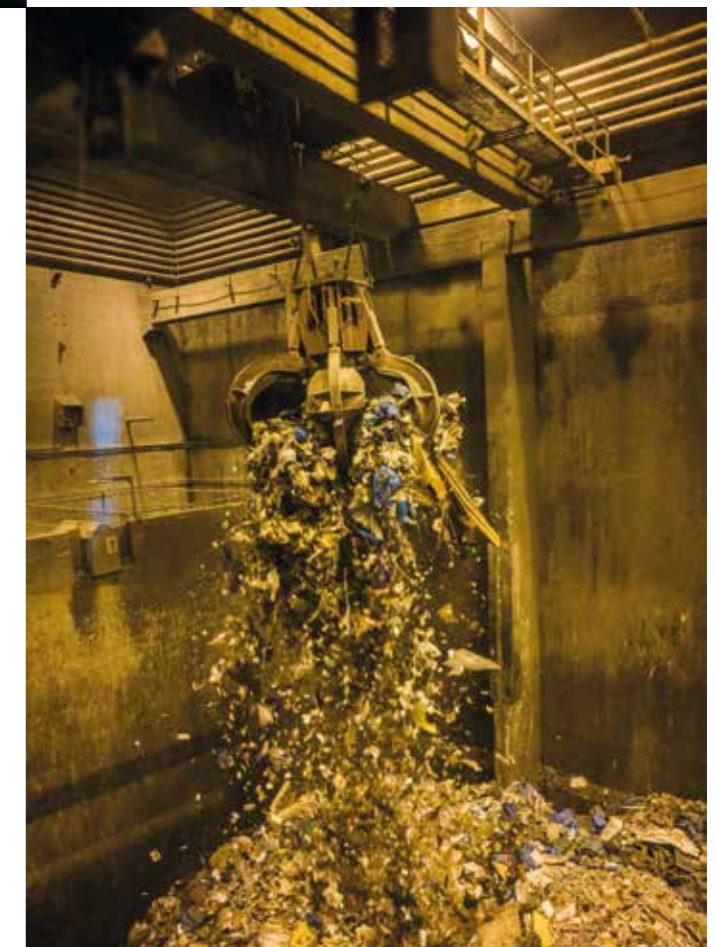
The grabber in the bunker transports the waste into the feeding hopper of the boiler
